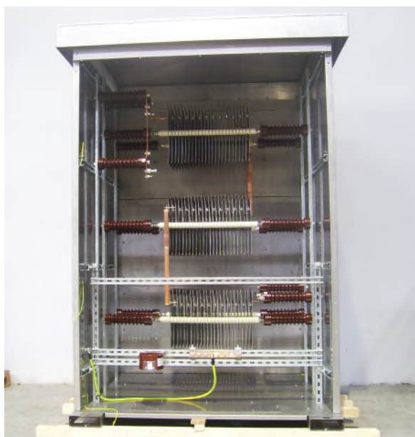
NOSPE-Widerstand 30 kV, 2000 A, 5 s NER 30 kV, 2000 A, 5 s
